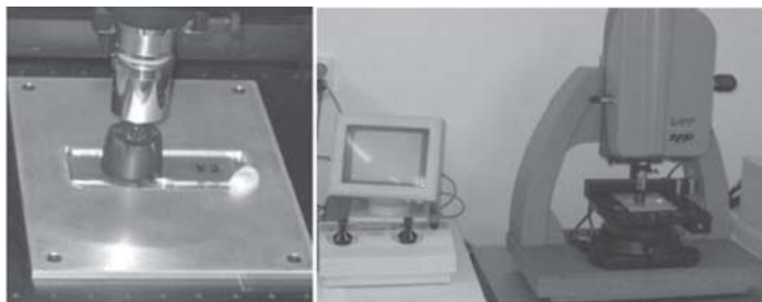
Fig. 13.20. Chocolate sample fixed to a microscope slide which fits onto the profilometry stage.
