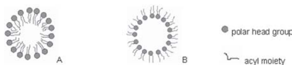
Fig. 11.13. Schematic representation of the H_I mesophase or micelle (A) and of the H_{II} mesophase or reversed micelle (B). Adapted from Savage & Dimick, 1995, and Sato & Koyano 2001.
